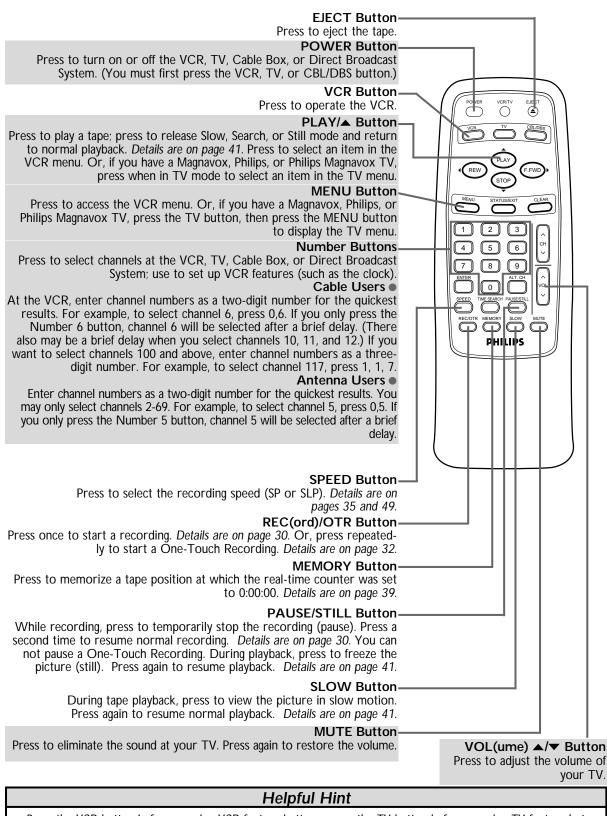
Press the VCR button before pressing VCR feature buttons; press the TV button before pressing TV feature buttons; press the CBL/DBS button before pressing Cable Box/Direct Broadcast System feature buttons.
